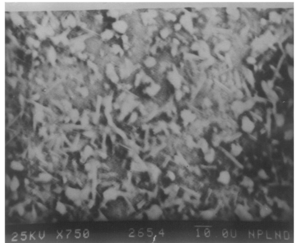
Figure 2 Scanning electron micrograph of typical yttrium-rich YBCO thin film. Needle-like structures may be noticed.
